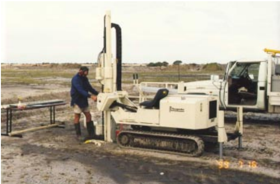
ABOVE: Effective sampling of acid sulfate soils is rarely a straightforward exercise but has become easier with the use of the Geoprobe, operated here by Ian Hall.
