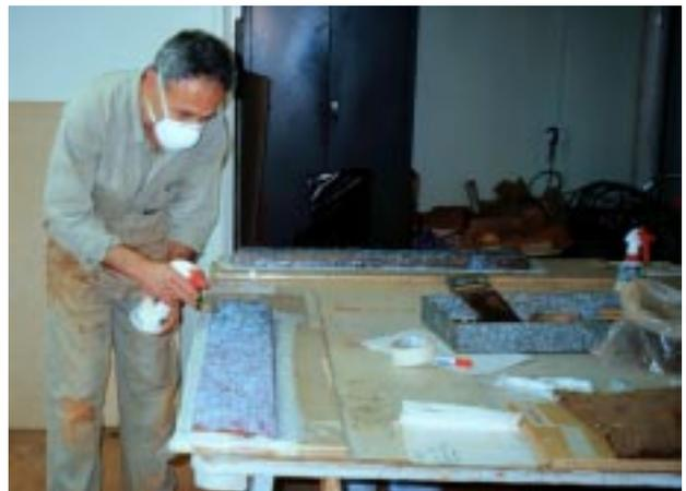
**Step 3 - The picked back soil profile is impregnated with the bonding solution.**
