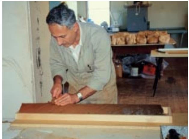
**Step 2 - The soil core is picked back to expose the natural features of the soil.**
