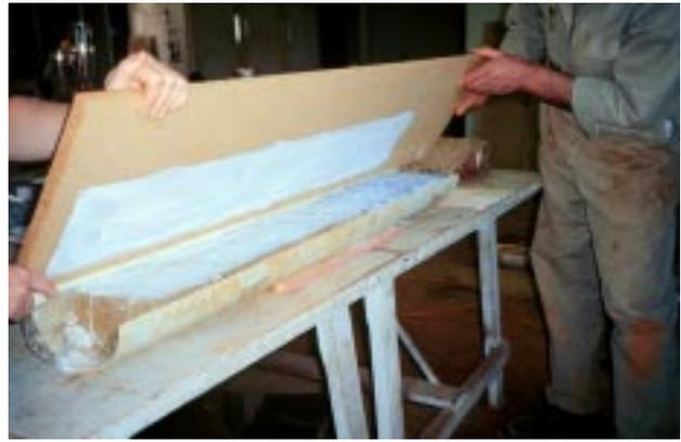
**Step 1 - The soil core is cut in half and glued to the backing board.**
