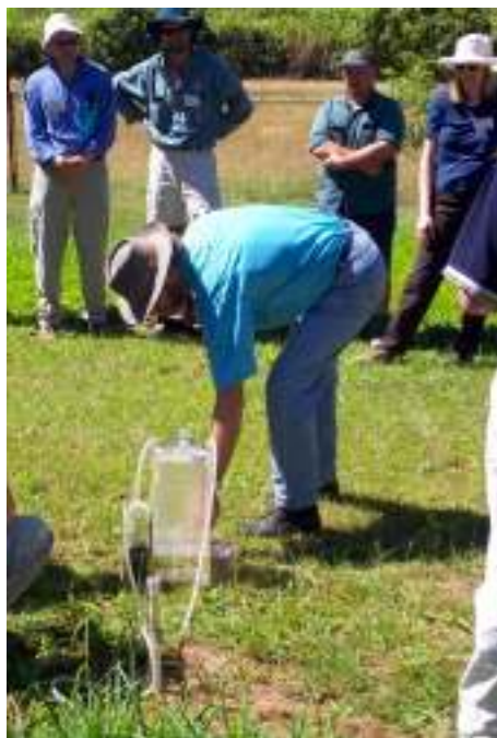
Photo 1: John Armour (NR&M) demonstrating how soil water samples are extracted from a depth of 1 metre below plots measuring changes in soil pH.
