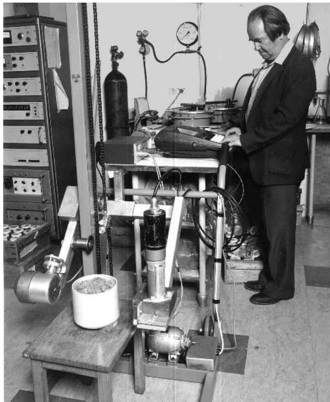
Cliff Gurr with the second model gamma ray soil column scanner built c 1975. Cliff is adjusting the AIM65 computer system (a contemporary to the Tandy TRS-80) controlling it. In those days nothing came off the shelf - even the instrument rack (rear left) was a leftover from the Blue Streak rocket program at Woomera. The scanner and soil core are in the foreground
